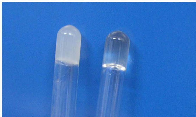
Fig. 5. The formed CS/GP and HTCC/GP hydrogels at 37 °C. Left: CS/GP hydrogel; right: HTCC/GP hydrogel.
